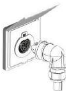
Figure 12 Wieland connector and specialised socket.
