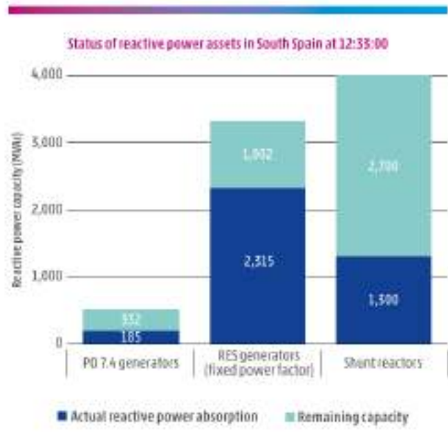
Figure 1-12: Capacity* of the different categories of reactive power assets in South Spain at 12:33:00
