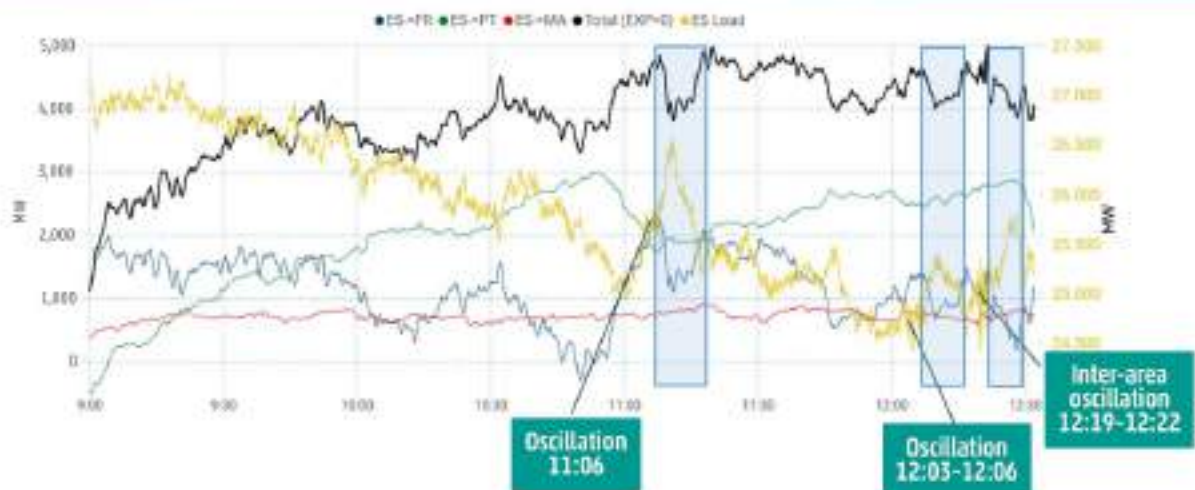
Figure 2-21: Spanish load and physical flows through ES-FR, ES-PT, and ES-MA between 9:00 and 12:32 (source: RE SCADA)
