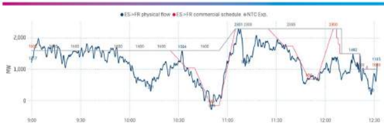
Figure 2-23: Commercial schedule and physical flow through the ES-FR border (source: RE SCADA)
