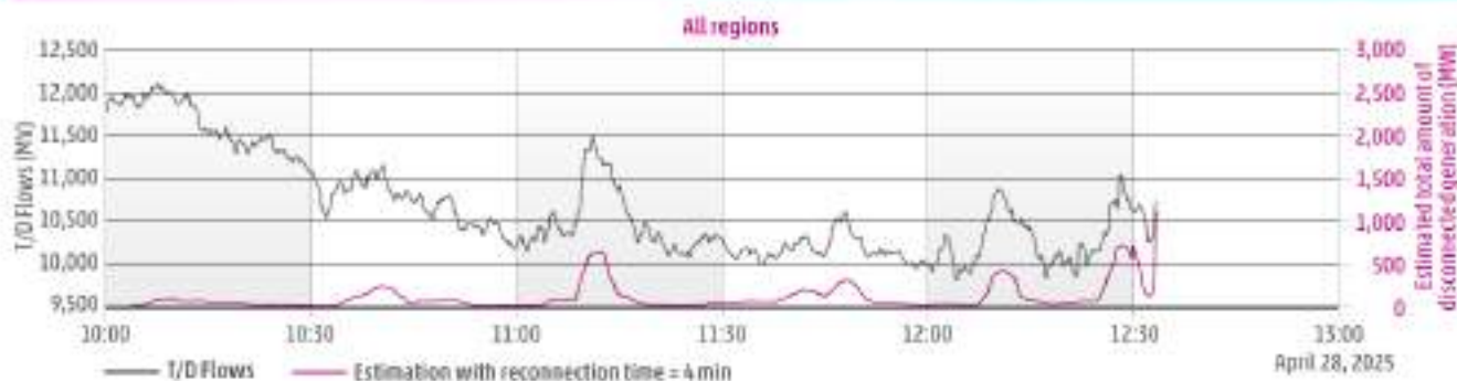
Figure 1-14: Correlation between the TSO-DSO flows and the estimated total amount of disconnected generation in Spain (units <1 MW connected to low-voltage grids)
