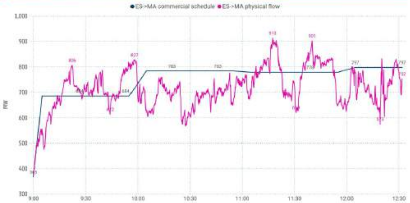
Figure 2-25a: Commercial schedule and physical flow through the ES–MA border (source: RE SCADA)
