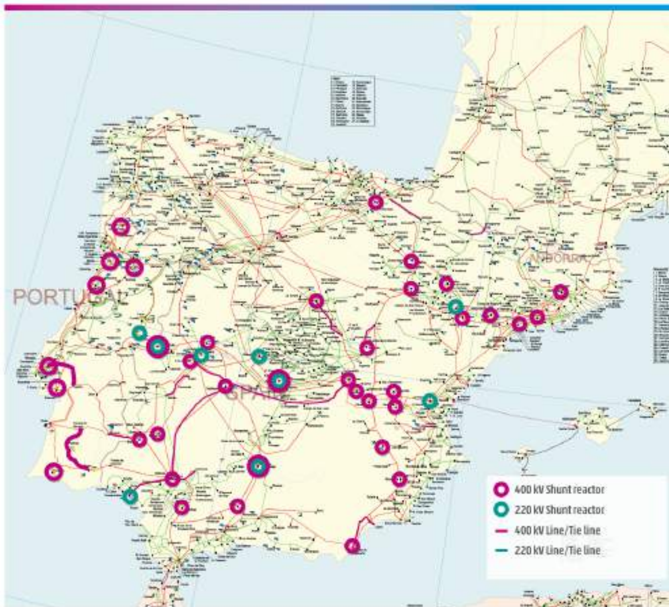
Figure 2-2: Iberian scenario: Open lines and reactances in Portugal and in Spain from 9:00 until 12:32
