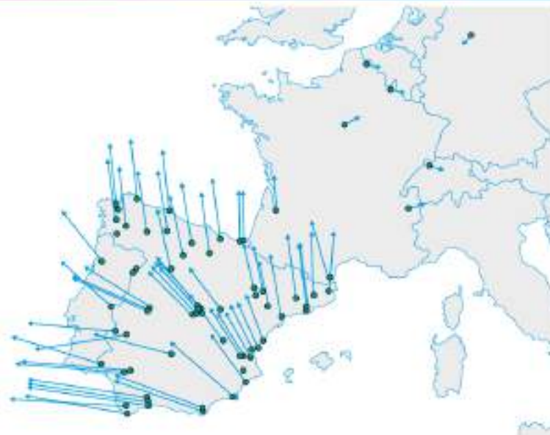
Figure 2-57: Mode shape of the 0.63 Hz oscillation (frequencies)
