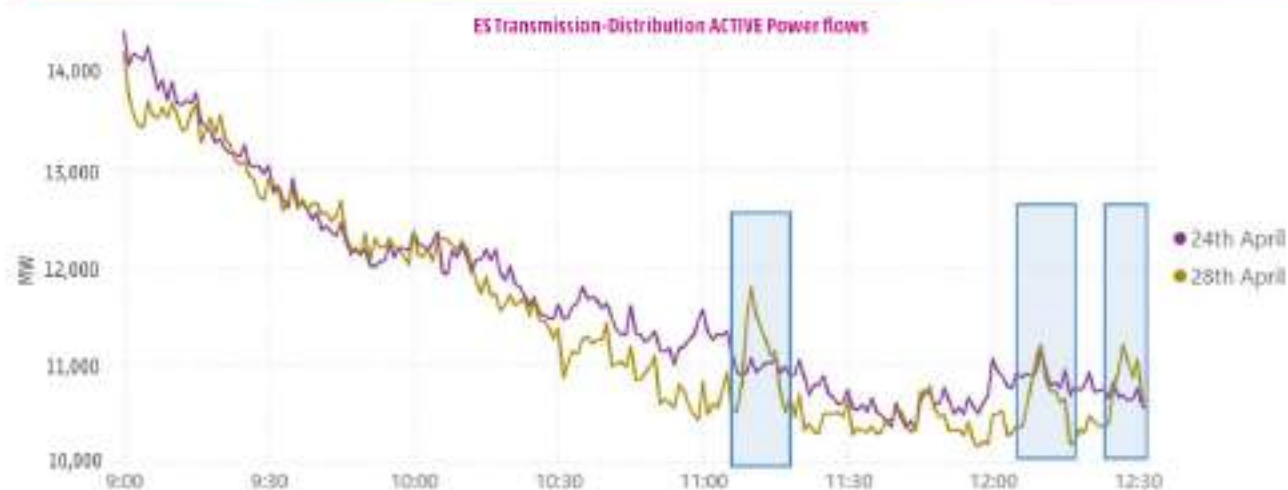
Figure 2-13: Spanish peninsula's transmission-distribution flows on 24 and 28 April between 9:00 and 12:32 (Source: RE SCADA)
