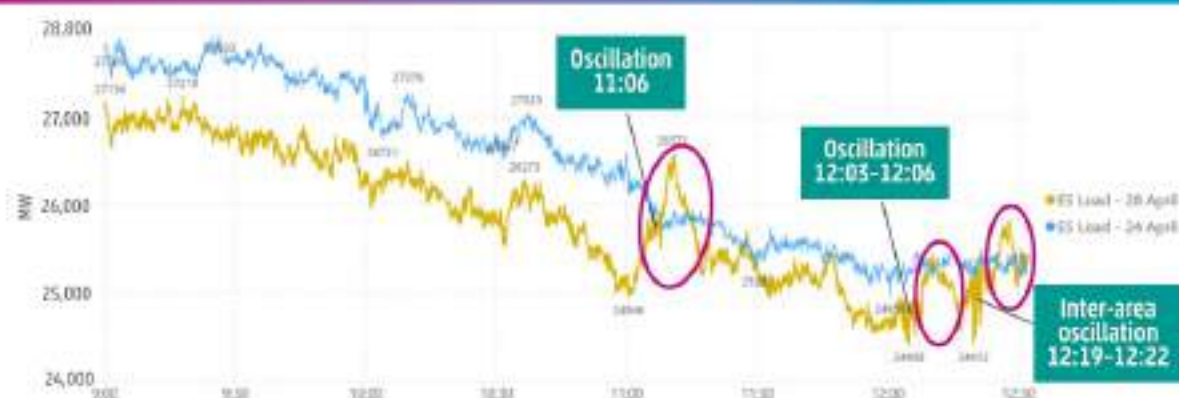
Figure 2-12: Total load in Spain on 24 and 28 April between 9:00 and 12:32
