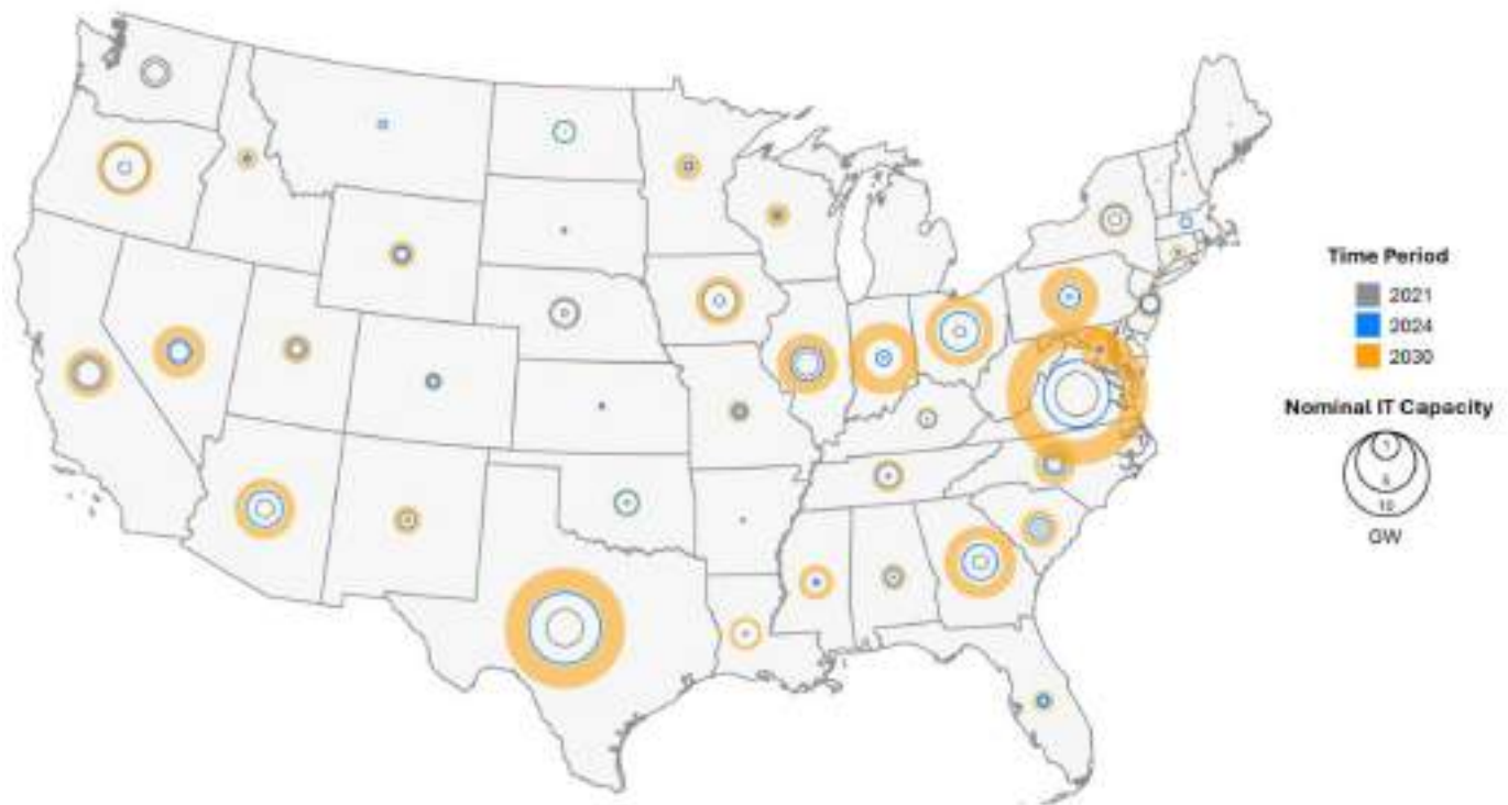
Figure 2. State-level data center nominal IT capacity (GW) today and in the planned 2030 pipeline. Inner circles show capacity in 2021 (gray) and 2024 (blue). Outer band shows scenario range of projected capacity in 2030 (orange). Circle area is proportional to nominal IT capacity. Estimates include small- and large-scale DC as well as cryptocurrency mining. Results highlight continued concentration in established markets (e.g., Virginia, Texas) alongside emerging growth in new states as developers diversify geographically.
